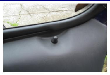
then angle it, about 10 o'clock, to feed the lock lever through the hole on the right. You might need to finger the lever a bit to attract it through the hole.
