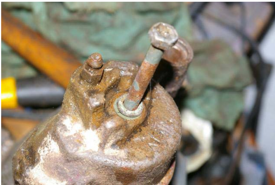
Figure 5. Removing the Piston
