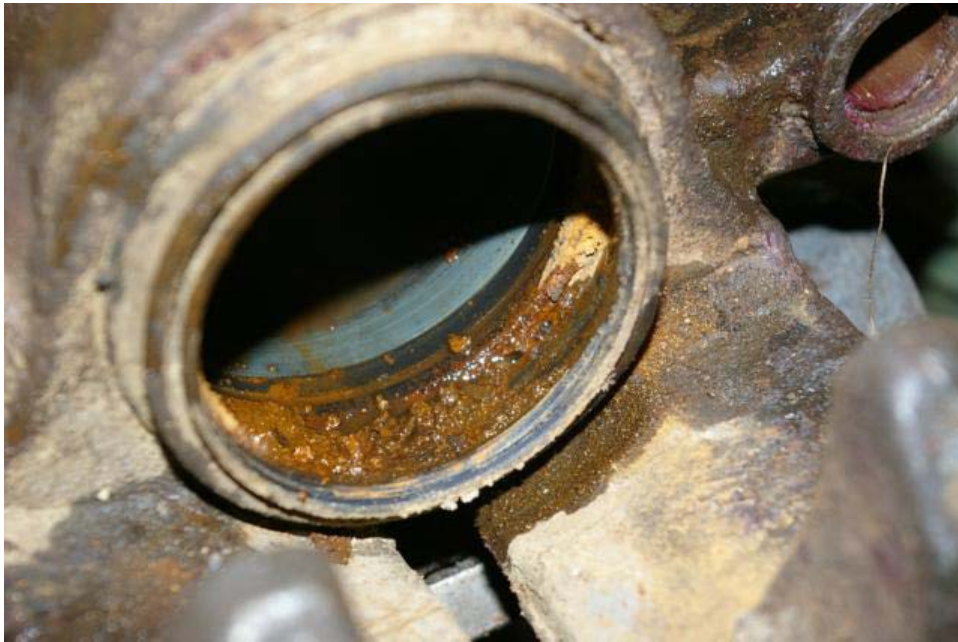
Figure 8. Dirt inside Caliper
