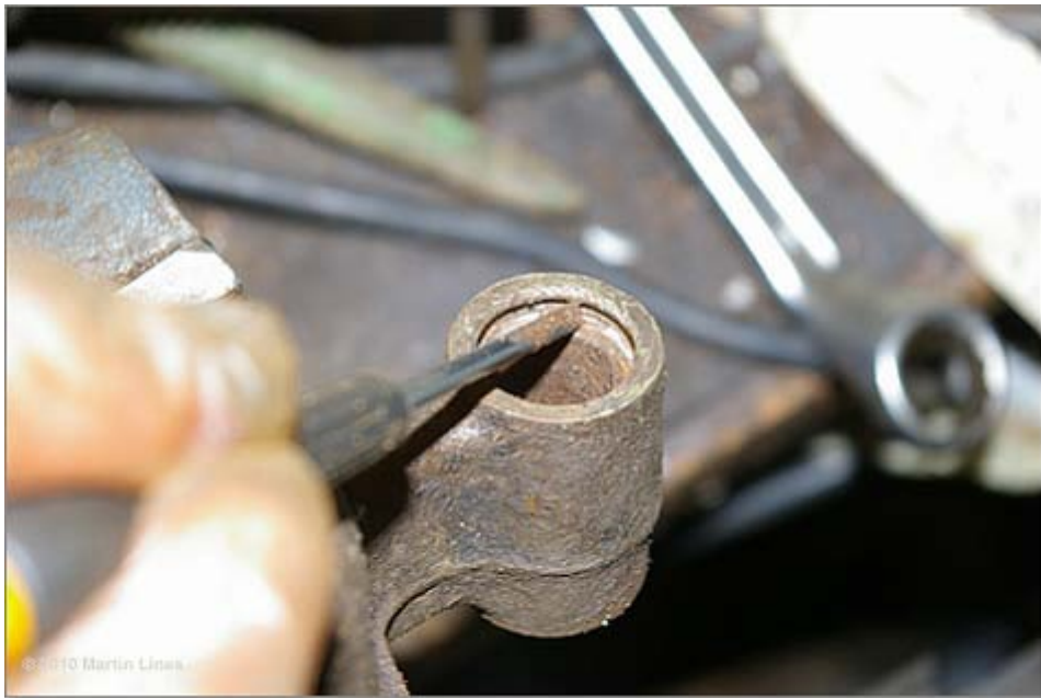
Figure 17. Cleaning the Caliper slider fittings
