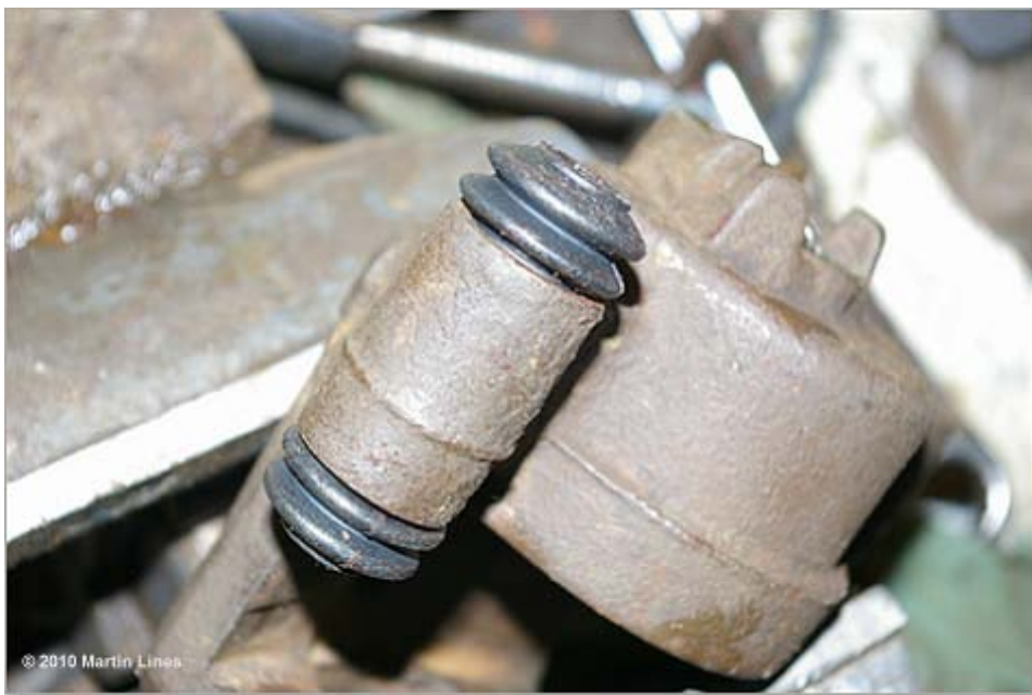
Figure 19. Fitting the boots
