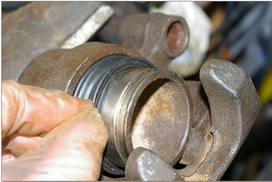
Figure 16. Stretching it over the Piston
