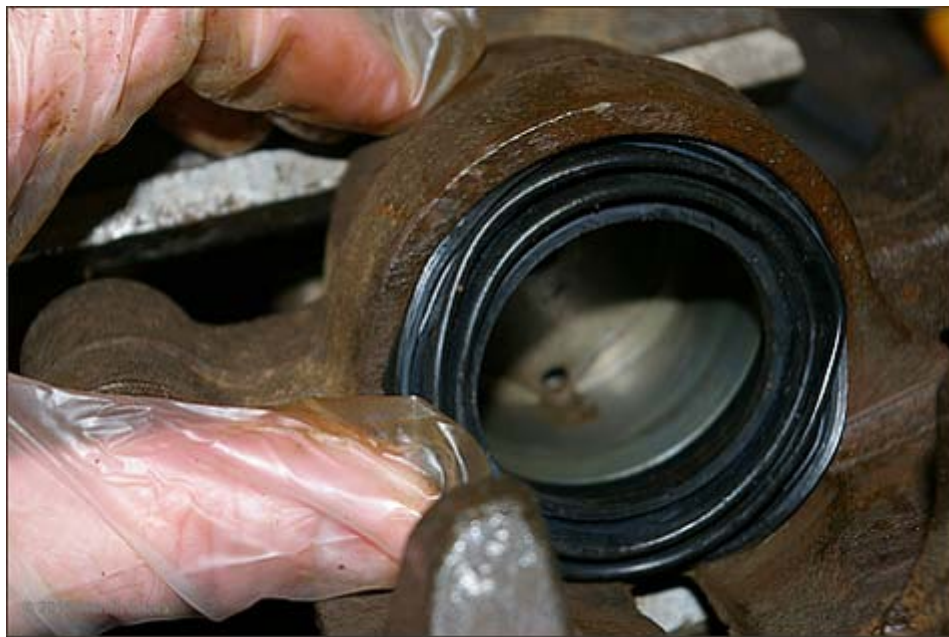
Figure 15. Fitting the Piston Boot
