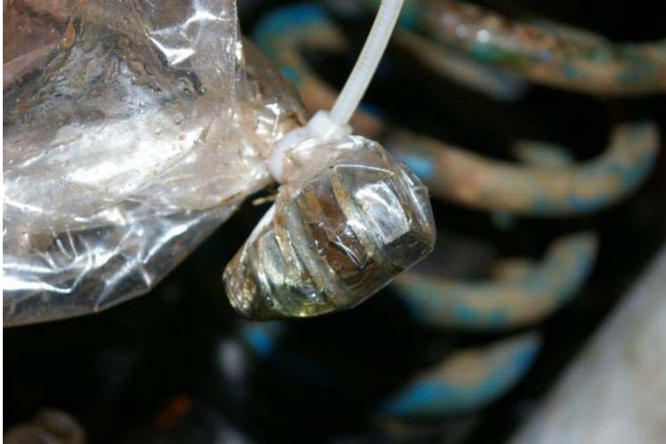
Figure 2. Sealing the Brake Pipe
