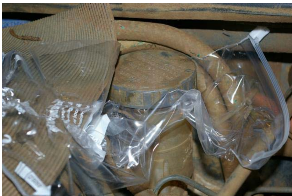
Figure 1. Sealing the Master Cylinder
