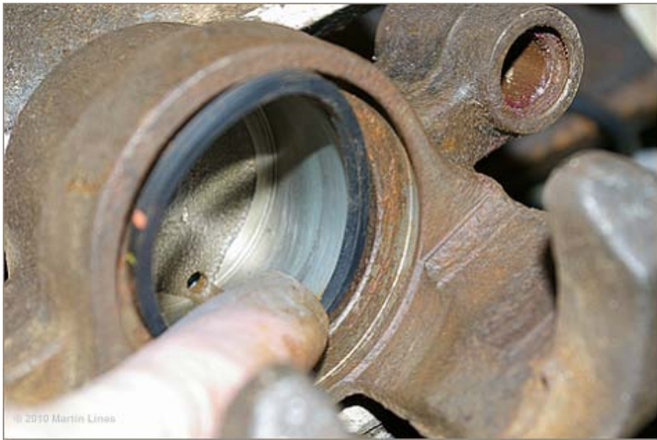
Figure 13. Fitting the seal
