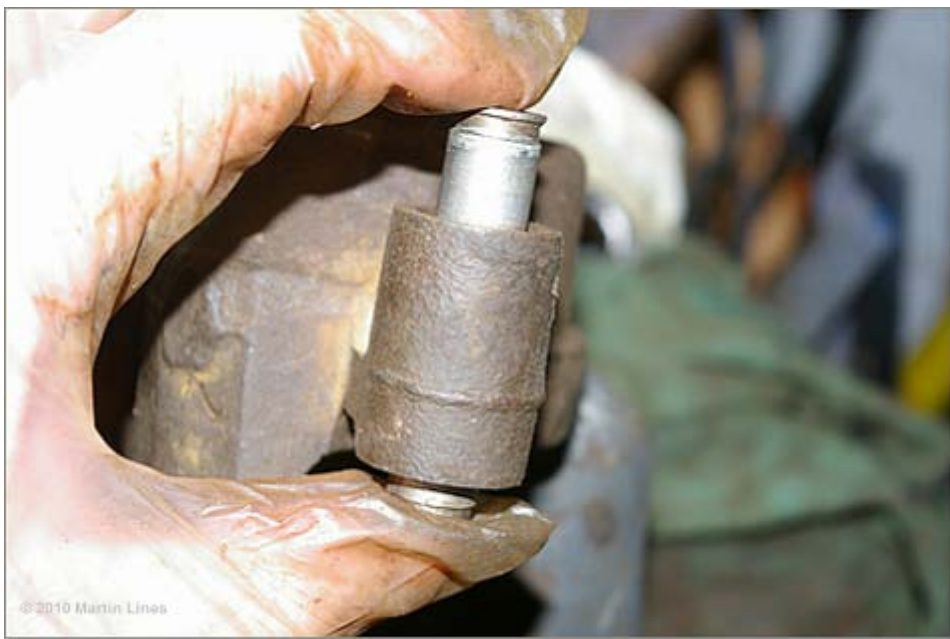
Figure 18. Checking the slider fit
