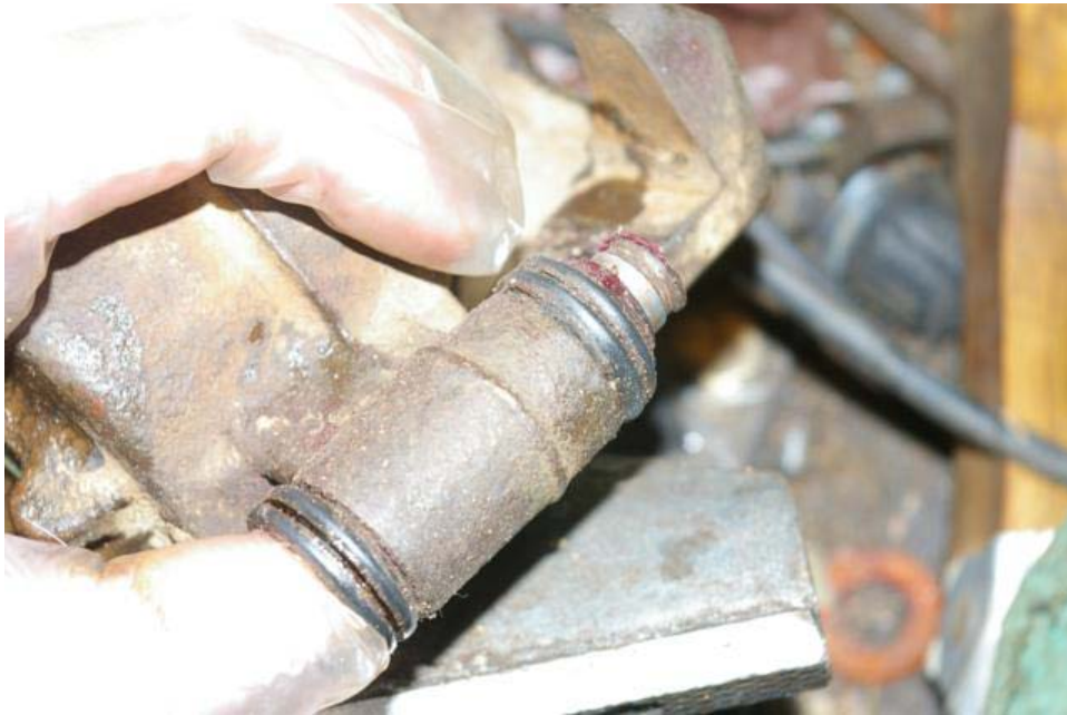
Figure 4. Removing the slider
