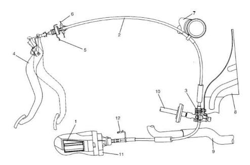
Simply prise of the cover (1) by using a large, flat bladed screwdriver.
