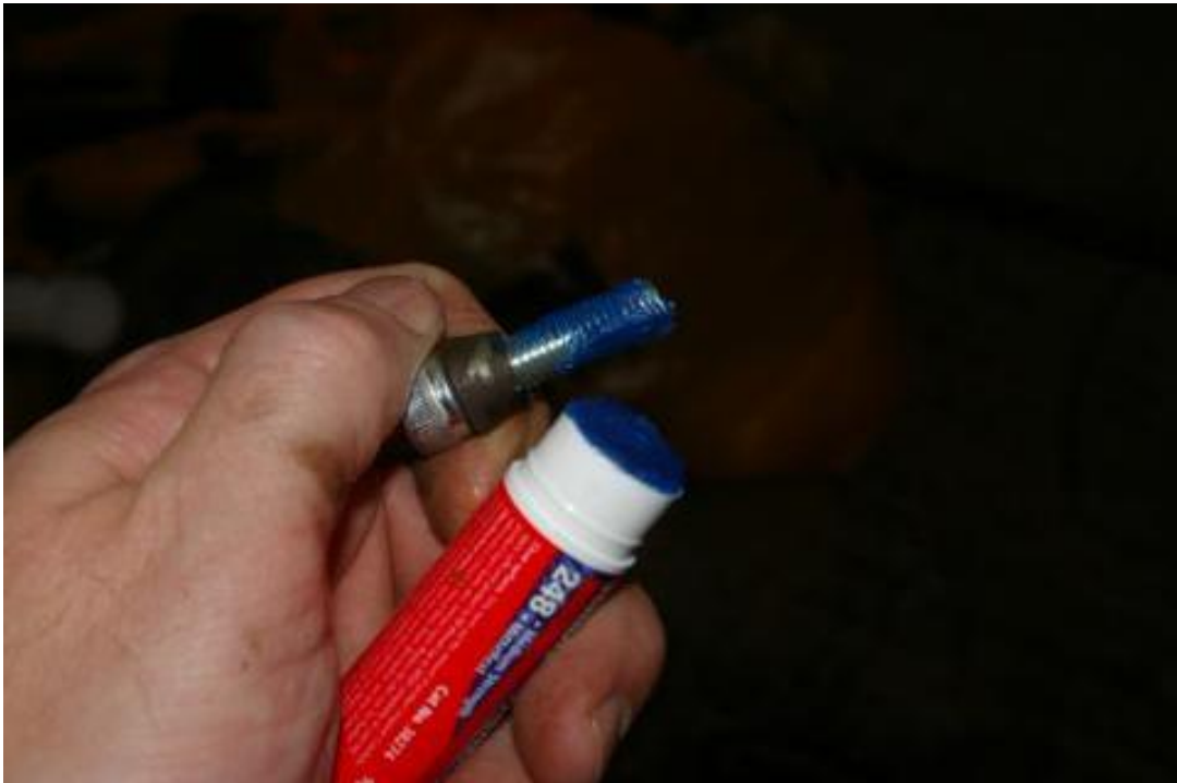
Figure 8. Coated bolt with thread locker
