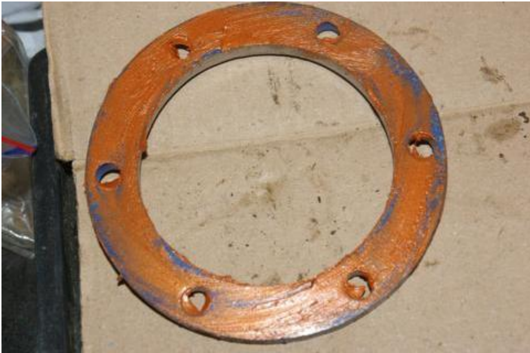
Figure 6. Spacer ring coated with sealant
