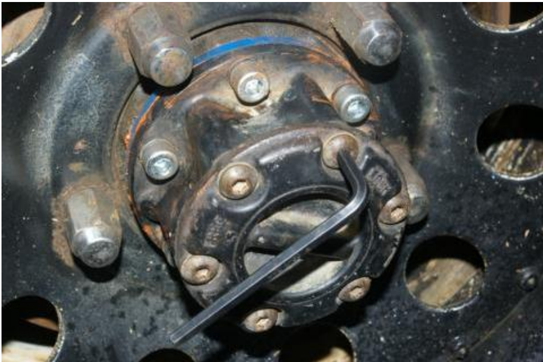
Figure 9. Removing the SJ Hub front plate
