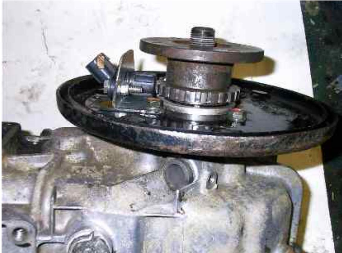
I cut away most of the backplate, leaving just enough to carry and protect the sensor.
