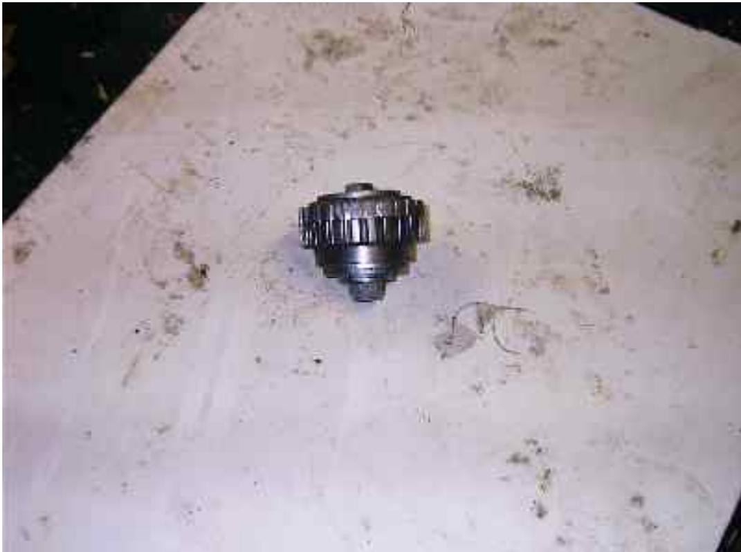
I unbolted the two gears. Then tack welded the gear to the rear TX box flange. There is a nice step in the flange which I butted the gear up to. This helped it to stay straight. I checked it was running true by fitting it to the TX box and spinning it round. When happy with it I welded it more securely.
