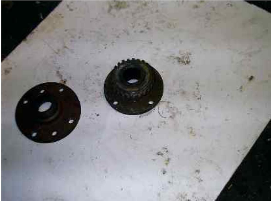
Next I used some car body filler to fill the gaps between the teeth. I also made it thicker to get it as close as possible to the TX box rear oil seal. I smoothed it off round and painted it! This was to keep the muck at bay.
