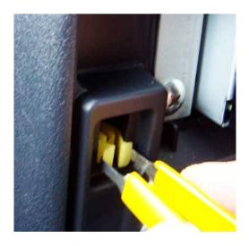
Here we have the rear of the trim panel with the clips attached, ready for refitting.
